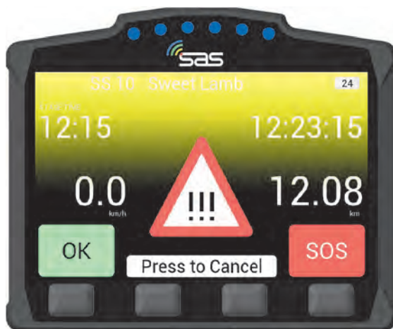
SCREEN 15. Manual Hazard in Transport Mode
