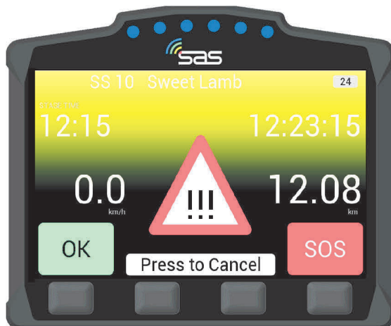
SCREEN 15. Manual Hazard in Transport Mode
