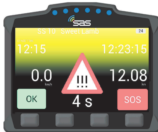
SCREEN 6. HAZARD Notification
