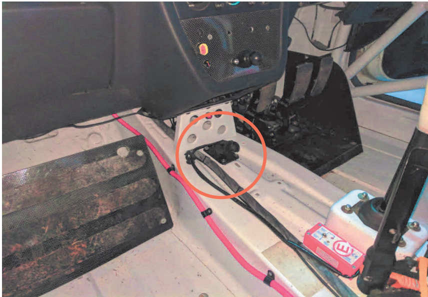
Figure 1. 25mm rubber ball securely attached to the tunnel
